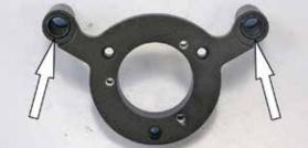
5. Install the four provided "O" rings into the K&N® base plate as shown.
