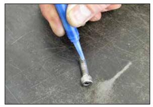
7. Apply one drop of the provided thread locker to the provided throttle body bolts.
